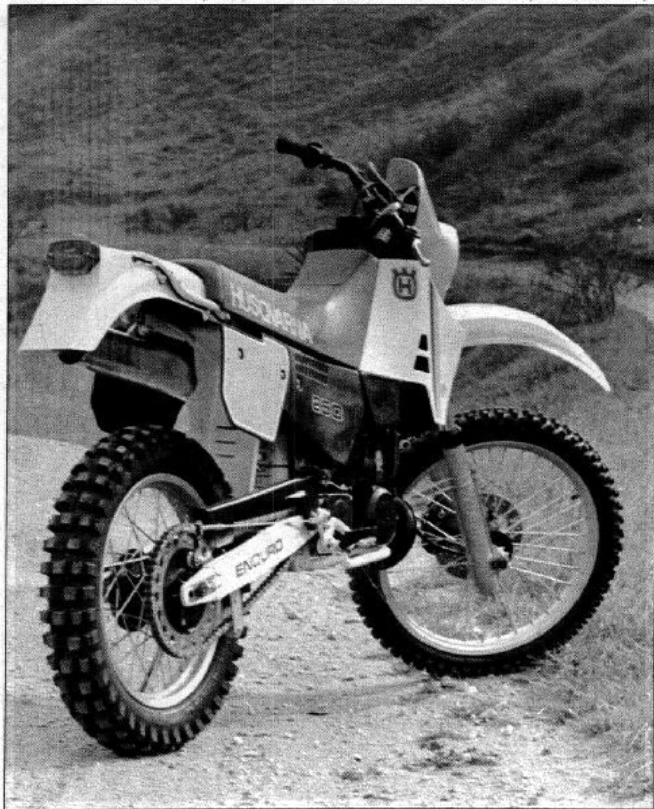
At 231 pounds dry, the Husky is a little on the heavy side. The black gas tank makes it hard to check fuel level.
